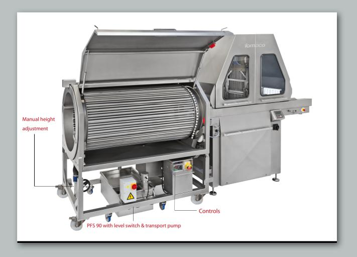
For our range of small to medium sized injectors we are please to introduce our compact continuous tumbler model CT 250, which includes a PFS 90 coarse filter with level switch and transport pump for collection of marinade/brine.
