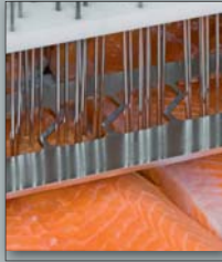
The unique needle bridge ensures an even and consistent injection level.
