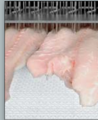
The injectors are specifically designed for processing of fish - preventing damage to the fragile fish meat structure.
