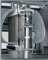
The unique needle bridge ensures an even and consistent injection level.
