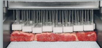
The sectionally divided pneumatic stripper feet prevent the product from moving when the needles are retracted.
